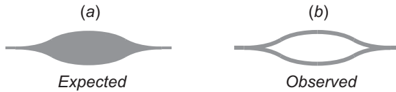
Fig 6.3 Expected (a) and observed (b) distributions of atoms in the Stern-Gerlach experiment.
